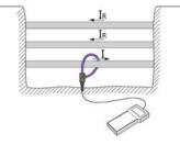
Place the flexcoupler around the cable that is to be identified or the phase in such a way that the arrow on the flexcoupler points towards the far end.
