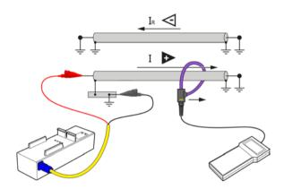
With the transmitter, current pulses with positive polarity are coupled to the cable that is to be identified. The coupled positive current pulses pass to the far end along the connected cable. On the other hand, the return current spreads to the earthed cable screens or to the other connected phases depending on the selected connection method and shows a negative polarity.
