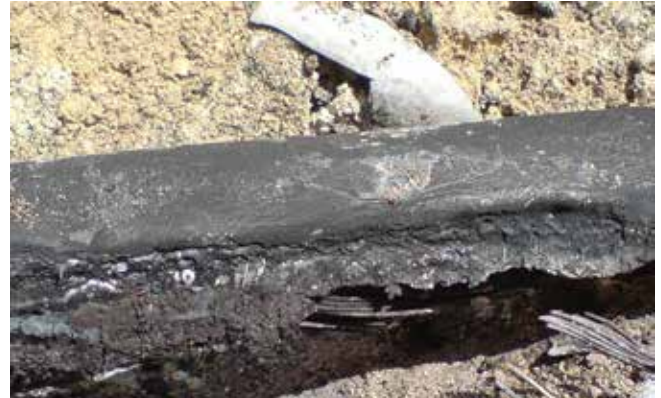
➤ vaporized core after cable fault, 132 kV XLPE
