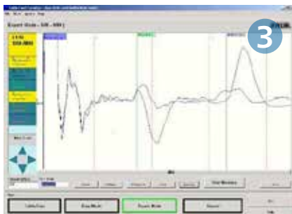
➤ SIM/MIM graph sequence IRG3000, display of automatically measured multiple sequence
