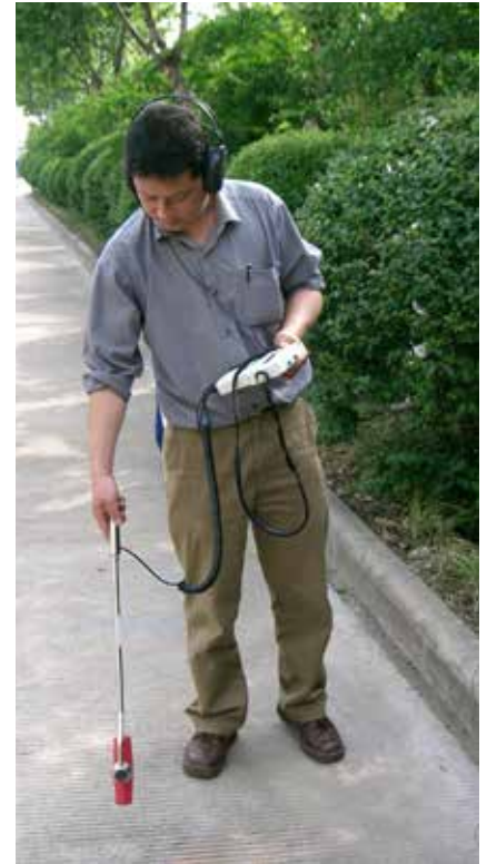
➤ detecting the twisted field signal
