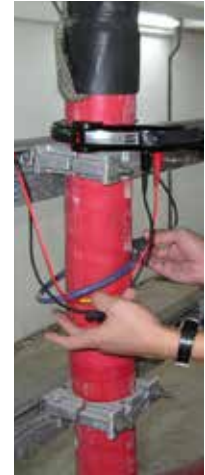
➤ accessible cable termination; calibration on full cable diameter
