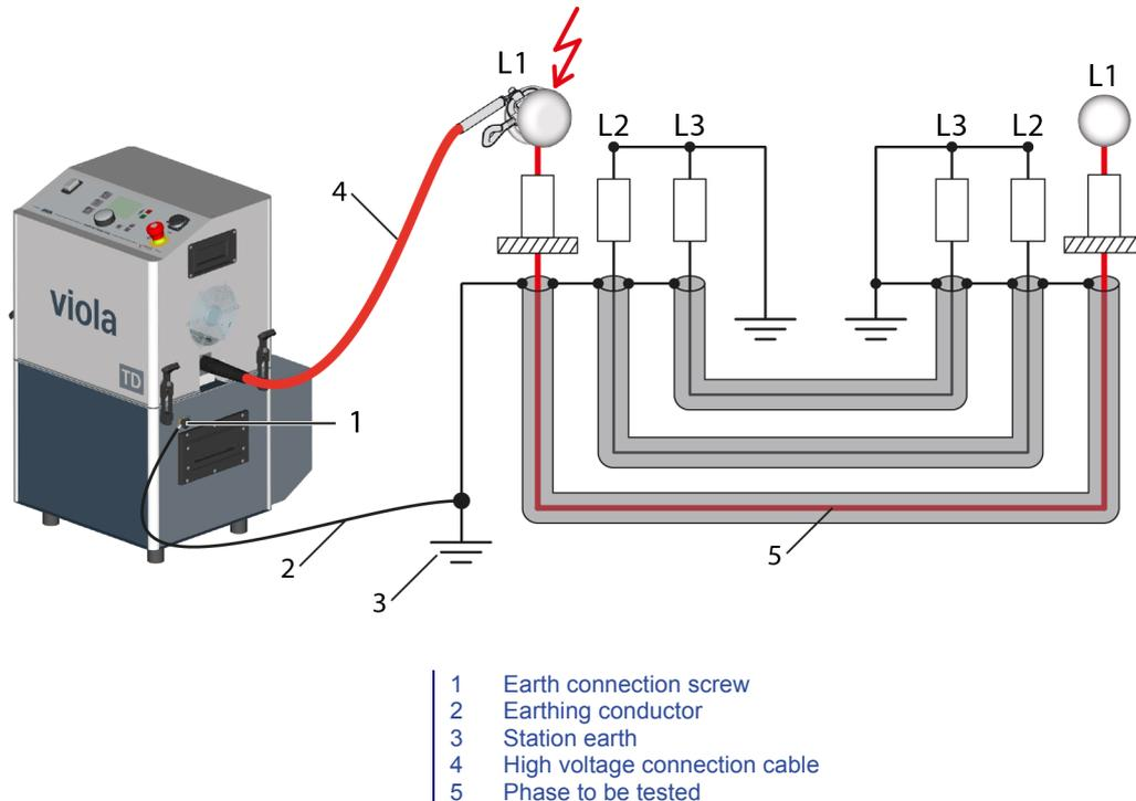
1. The scope of delivery of viola TD comprises an earthing conductor. Connect the earthing conductor to the station earth.
