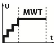
In the MWT stage the proper cable test is carried out with a continuous dissipation factor measurement at a defined test voltage (e. g.  $2 \times U_0$ ).
