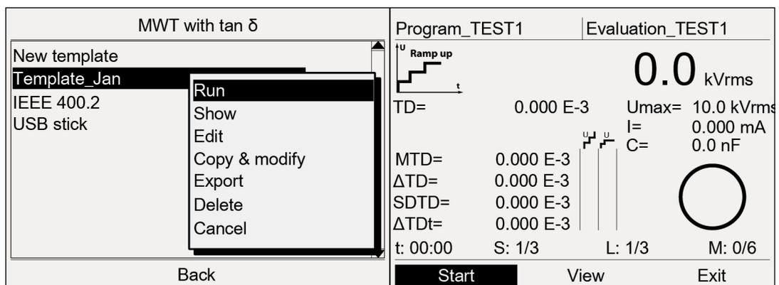
5. Make your selection in the lower menu bar *Start* and press the rotary knob to confirm.
