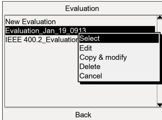
2. In the menu *Evaluation* select an evaluation and press the rotary knob to confirm.
