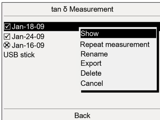
If a measurement is not complete, – that is, not all phases are measured or the measurement was cancelled –, the respective log is indicated by a cross. You can start the cancelled measurements directly from the menu *Logs* and complete the same. For this purpose, select the respective log and, in the context menu, select the menu item *Continue measurement*. This menu item is shown, if you have selected a previously cancelled measurement.
