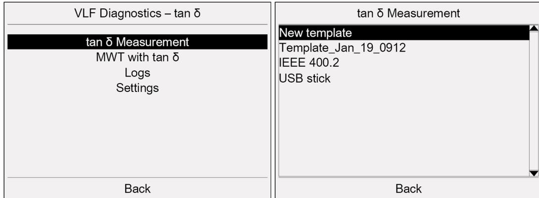
3. In the menu *tan-δ Measurement* select the menu item *New template* and press the rotary knob to confirm.
