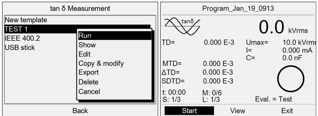
5. In the lower menu bar, select *Start* and press the rotary knob to confirm.
