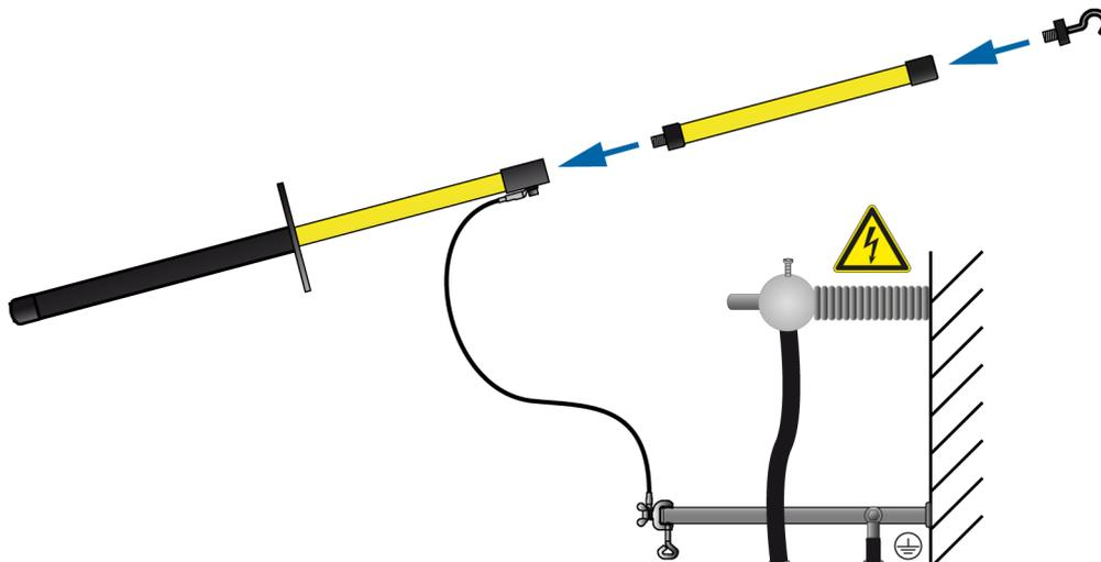
3. Use the black handle to hold the discharge and earthing rod and contact the test object with the tip of the discharge and earthing rod.
