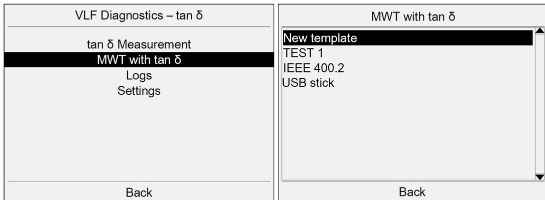
3. In the menu *MWT with tan δ* select the menu item *New template* and press the rotary knob to confirm.
