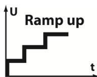
In the ramp-up stage, the test voltage is built up. During this time, a dissipation factor measurement is carried out on the test object for pre-defined voltages (e. g.  $0.5 \times U_0$ ,  $1 \times U_0$  and  $1.5 \times U_0$ ). For each voltage step, 6 to 10 measured values are recorded. The measurement results provide information on the actual condition of the cable and allow the subsequent cable test to be adapted to that cable condition.
