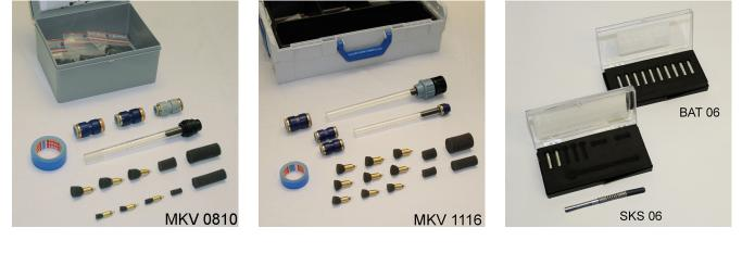
The calibration sets MKV 0810 and MKV 1116 in conjunction with the accessory micro- transmitter SKS 6 (code-no. 231941) are destined for the calibration of subducts with an internal diameter 8,0 to 16,0 mm. The calibration can be done for single subducts as well as for multi subducts. By the calibration defects or blockages on the subducts can be detected in advance thus a good blowing-in performance can be achieved.
