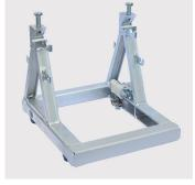
Steel rope drum alone, divisible for coiling cords, ropes or cable rings, suitable to pilot rope winches SBS 510 and SES 410. Dimension D 410/100x210 mm, for rope up to 1100 m D 4 mm, or 750 m D 5 mm. For coiling rings there will be mounted 3 segments into the drum. With this mounted steel segments the capacity will be reduced to app. 900 m D 4 or 500 m D 5 mm.
