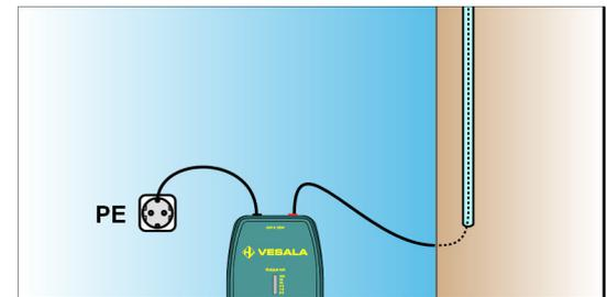
**Receiver:** Scan wall surface with the LA43 probe to track a signal minimum between two strong signals. If the cable is further away than 30cm, use SA43 probe instead.
