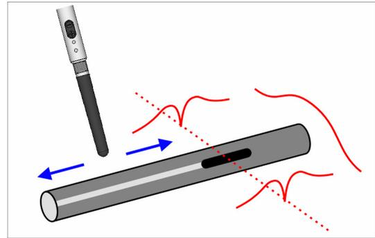
**Task: The route of a non-conductive tube needs to be traced inside a wall.**
