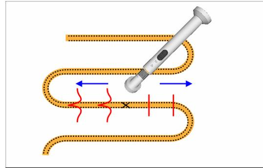
**Task: An open fault (cut) in a floor heating cable needs to be traced.**
