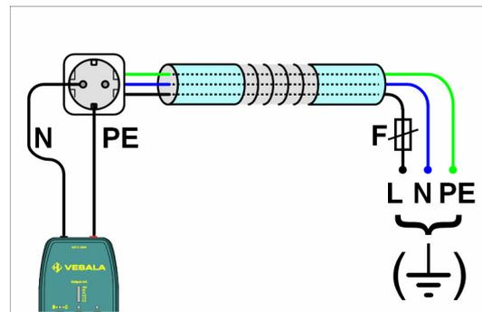
**CL43:** Use LA43 probe. Trace the cable route by following the signal maximum. Right above the cable there is often a signal minimum.
