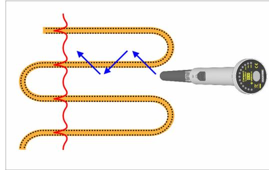
**Task: A short circuit in a floor heating cable needs to be traced.**
