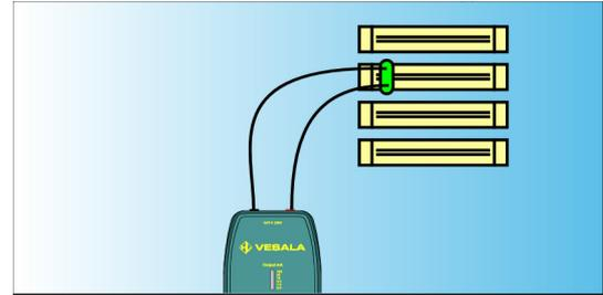
**Receiver:** Use KA43 probe and scan as close as possible over terminal modules to find signal maximum. Strongest signal is above the right pair. Due to cross talk, signal can be heard elsewhere too but weaker.
