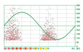
Example: Phase-resolved display of a partial discharge activity at 0.1 Hz
