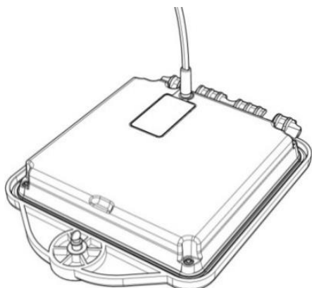
Figure 4.13 Charging the transmitter Li-ion battery pack
