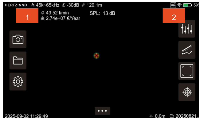
3.1.2-Gas Leakage Detection Interface
